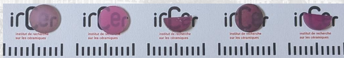
Photograph of 10-mm-diameter \text{Al}_2\text{O}_3\text{:Cr} ceramic samples containing 0.1 to 0.5 molar percent chromium, arranged in descending order of chromium content from left to right (0.5 molar percent on the right and 0.1 molar percent on the left). The samples were sintered using the SPS method at 1,400 °C for 15 minutes under a pressure of 130 MPa.
