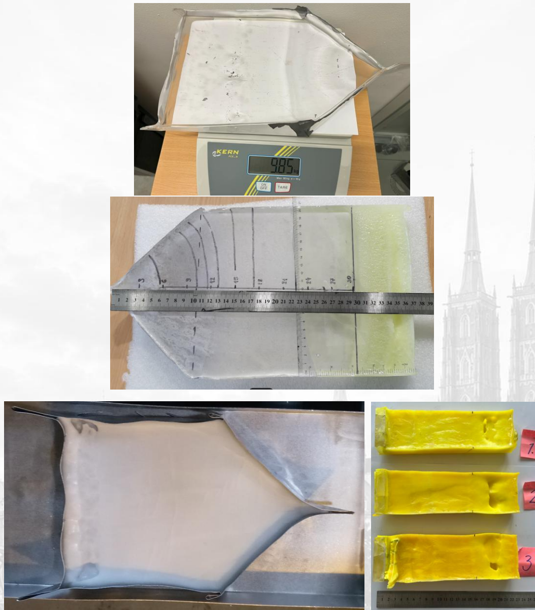
Fig. 1: Sapphire, YAG crystal and eutectic ceramic grown via HDC method.
